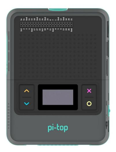
The miniscreen of the pi-top [4] can be found on the front, comprised of an 128x64 pixel OLED screen and 4 programmable buttons.
