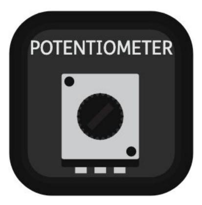
Note: This is a Analog Component which connects to a Analog Port [A0-A3].
