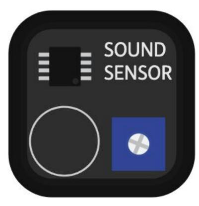
Note: This is a Analog Component which connects to a Analog Port [A0-A3].
