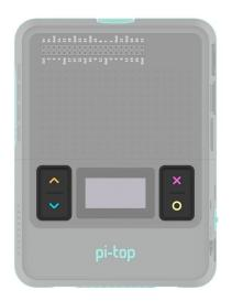
The miniscreen's buttons are simple, and behave in a similar way to the other button-style components in this SDK. Each miniscreen button can be queried for their "is pressed" state, and also invoke callback functions for when pressed and released.
