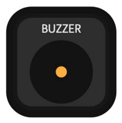
Note: This is a *Digital Component* which connects to a *Digital Port* [D0-D7].
